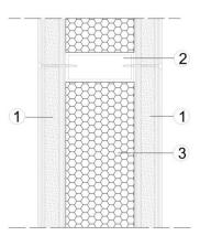
Detail of a partition with Yesograf on both sides (1), metalic or wooden strip as an structure (2) and insulation between boards (3). Preferably placed when it is dry.
