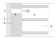
Detail of a board with gypsum and Yesograf (I) front (2). It is installed in the outer side of the ceramic brick (3) or in another material, and the insulation (4) strips (5) or metalic brackets or made of another resistant materia, fixed on the front (6) where the board is srcrewed (7). Preferably placed when it is dry.
