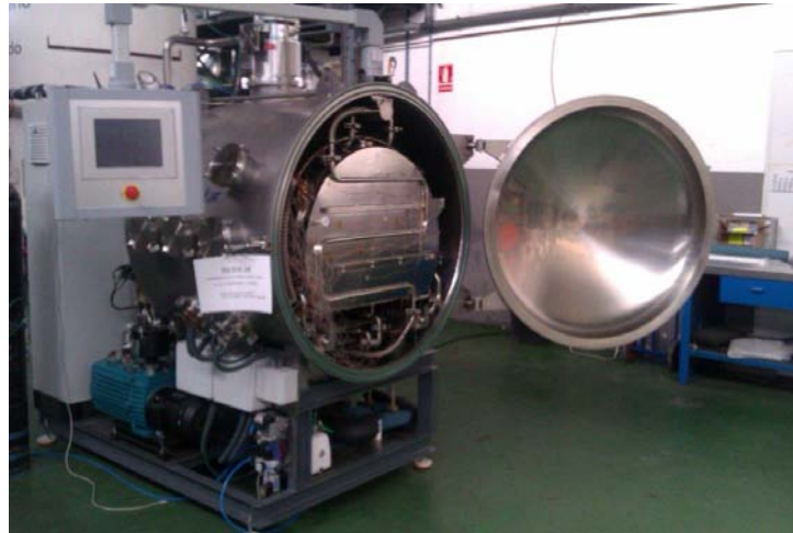
Figure 36. Thermal Vacuum Chamber at the IDR
