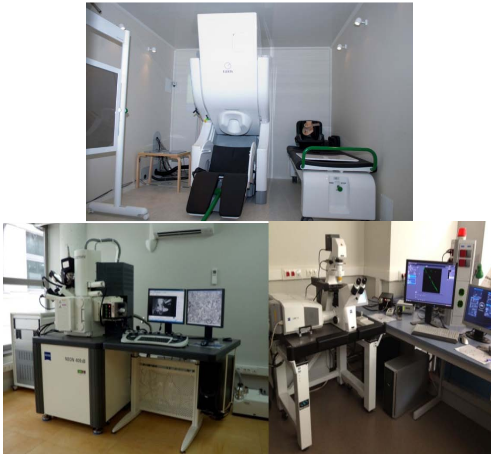
Figure 26. CTB Equipment: a) Magneto-encephalography system and b) double-beam microscopy system (agreement with Zeiss)
